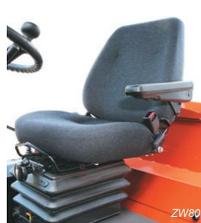
A long-stroke suspension seat, which absorbs shocks and vibration well, is standard.
