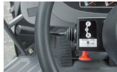
If the forward/reverse lever is not in neutral (N), the engine cannot start.
