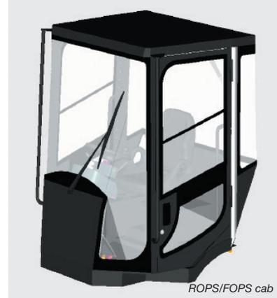
The ROPS/FOPS cab is adapted to protect the operator from roll-over accidents and falling objects.
