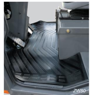
The walkthrough type cab allows for easy access from either side. The flat floor enables easy cleaning.
