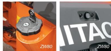
The fuel cap and engine cover can be locked with the engine key.
