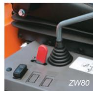
The control lever and auxiliary function lever lock for safety.
