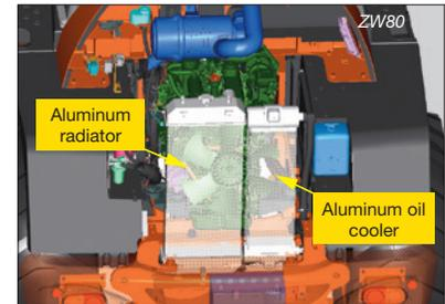
The aluminum radiator and oil cooler are located side by side for easy cleaning.
