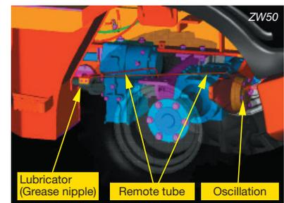
Remote easy access lubrication and engine oil drain.
