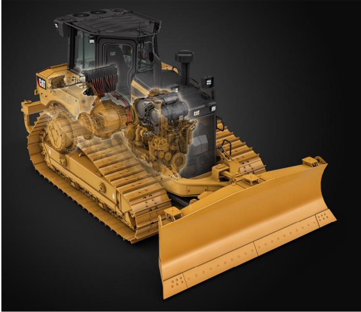
The new Cat® D6 XE is the world's first high drive Electric Drive dozer. It reflects more than a decade of experience and continued Electric Drive development for track-type tractors and other machine families. Because of ongoing advances in design and proprietary testing, today's refined Electric Drive power train is even more simple, efficient and robust.
