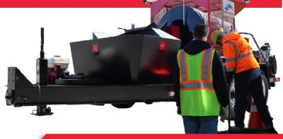
When using our Mixer, you can heat 650 lbs of material to 350°F in less than 10 minutes. No runs to the asphalt plant, no material costs & no waste. The Mixer can also recycle chunks of old raw road material.
