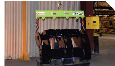
Durable composite lifting equipment can be used in industrial applications such as manufacturing earth moving equipment
