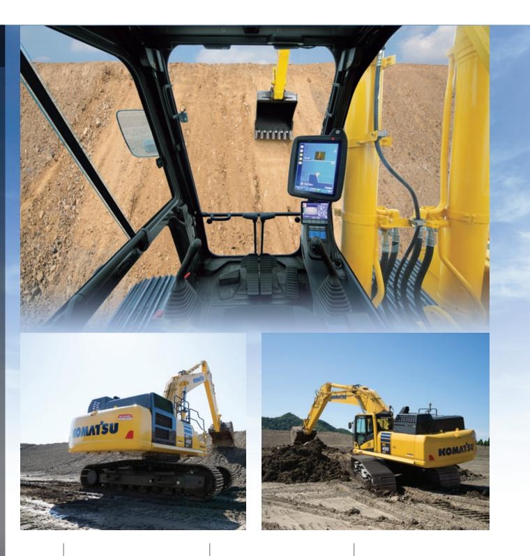
**NET HORSEPOWER** 359 HP @ 1900 rpm 268 kW @ 1900 rpm **OPERATING WEIGHT** 105,670–107,850 lb 47930–48920 kg **BUCKET CAPACITY** 1.47–4.15 yd<sup>3</sup> 1.12–3.17 m<sup>3</sup>
