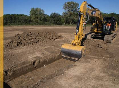
Cat® GRADE with Assist brings grading speed and accuracy to a new standard by automating boom and bucket movements typically achieved by the operator. This significantly reduces manual inputs, errors, and fatigue—improving grading consistency for operators at all experience levels.
