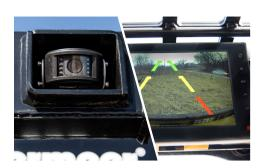
**REARVIEW CAMERA WITH IN-CAB** MONITOR. An in-cab monitor provides added visibility, enhancing maneuverability.
