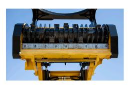
**ABOVE-GROUND MULCHER - RINGED ROTOR.** The ringed rotor design of the above ground mulcher head attachment helps guide material into the path of the cutting tips for effective single-pass clearing and full-tip coverage. By controlling the depth of cut, the engine can be loaded to peak operating performance.
