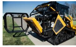
**ENGINE ENCLOSURE.** Engine compartment doors provide convenient access to maintenance points.
