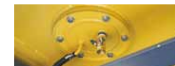
Fuel Drain Valve
