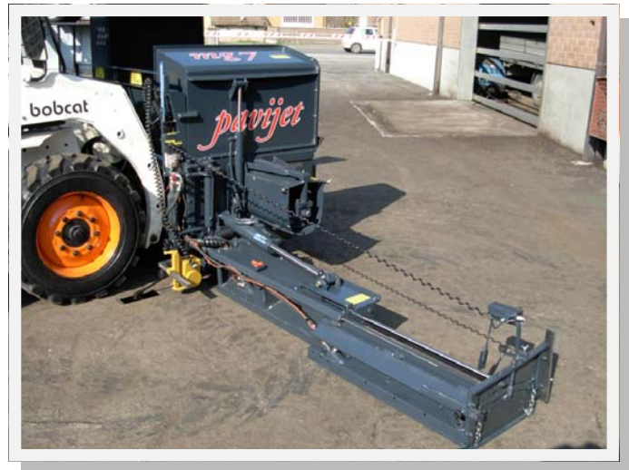
MG7 screed extended to its full width. Screed can also be heated for use with hot bitumen.
