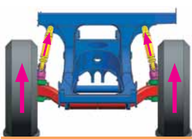
BOTH STRUTS IN COMPRESSION WITH NO HORIZONTAL DEFLECTION
