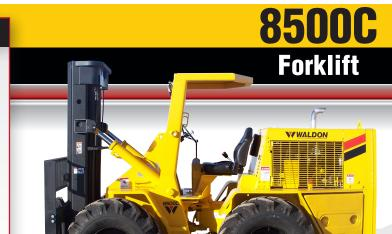
pallets up 34% grades, through sludge, mud or snow: operate in standing water with full braking capacity, clear low 8 foot obstructions, go in boxcars - there just isn't a more productive 12,000 lbs. capacity forklift available!
