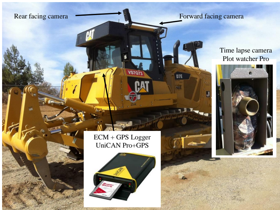
Figure ES-3 Activity measurement setup on the Caterpillar D7E hybrid
