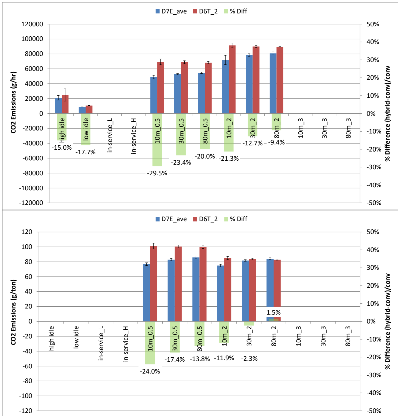
Figure 6-1 CO 2 Emissions on a g/hr and g/ton basis for the different controlled push tests D6T.
