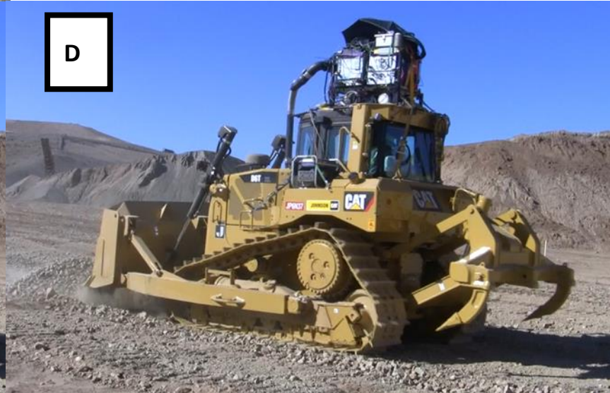
Figure 5-3 D6T bulldozer pushing a single 13 ton full load pile 30 meters
