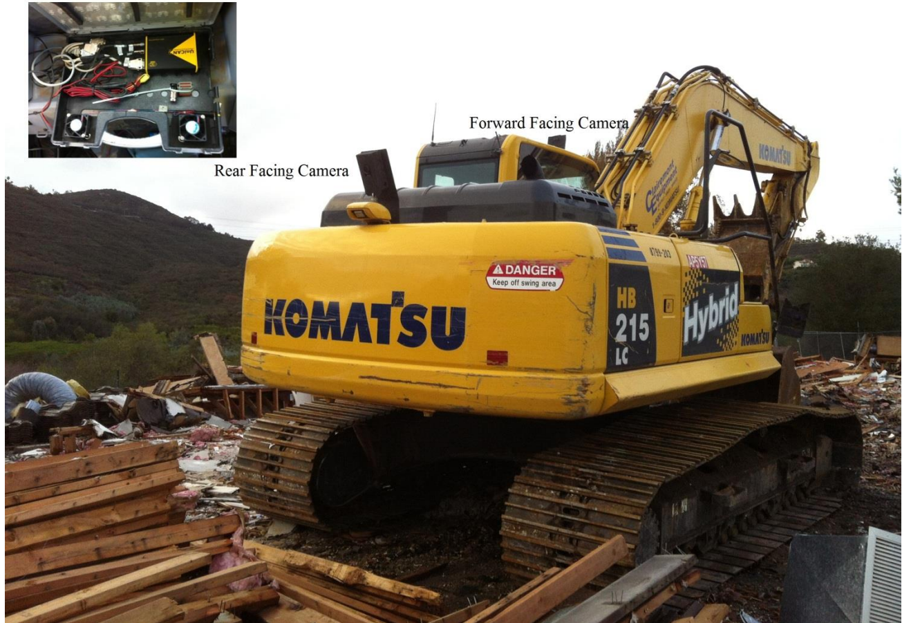
Figure 3-5 Activity measurement tools, ECM, GPS, and time lapse video on the HB215.
