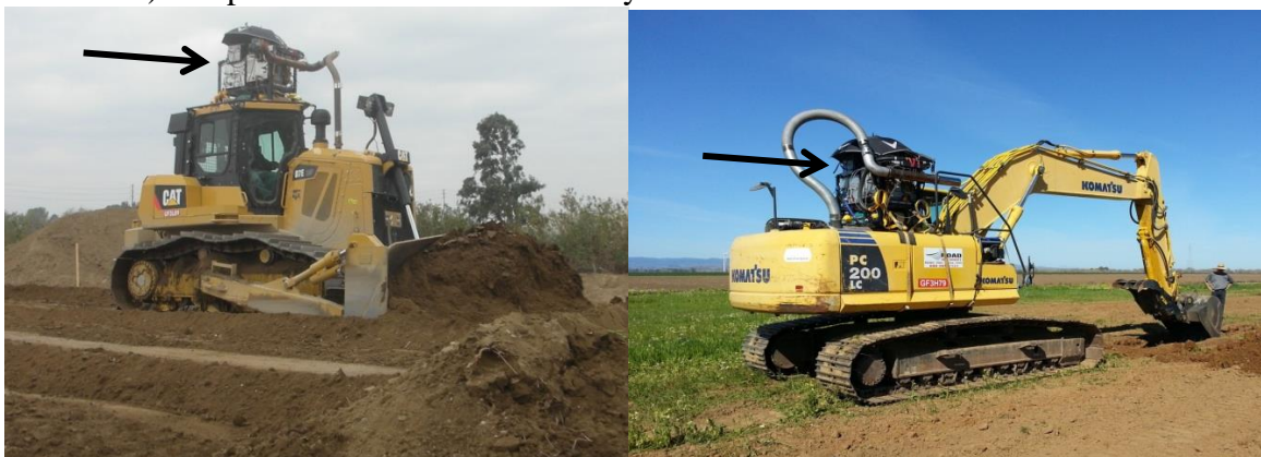
Figure ES-7: PEMS in-use measurement example for the bulldozer and excavator units
