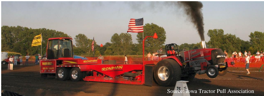
Figure 5-12 Typical tractor pull approach for evaluating tractor performance
