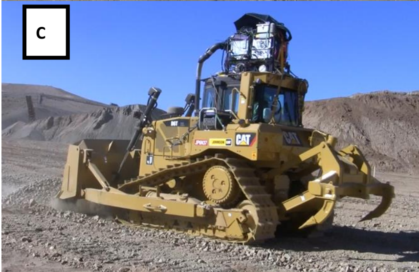
Figure 5-3 D6T bulldozer pushing a single 13 ton full load pile 30 meters
