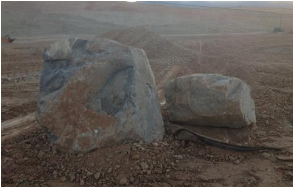
Figure 5-11 Pushing large heavy objects as an alternative to pushing piles (7.5 and 3.5 ton rocks)
