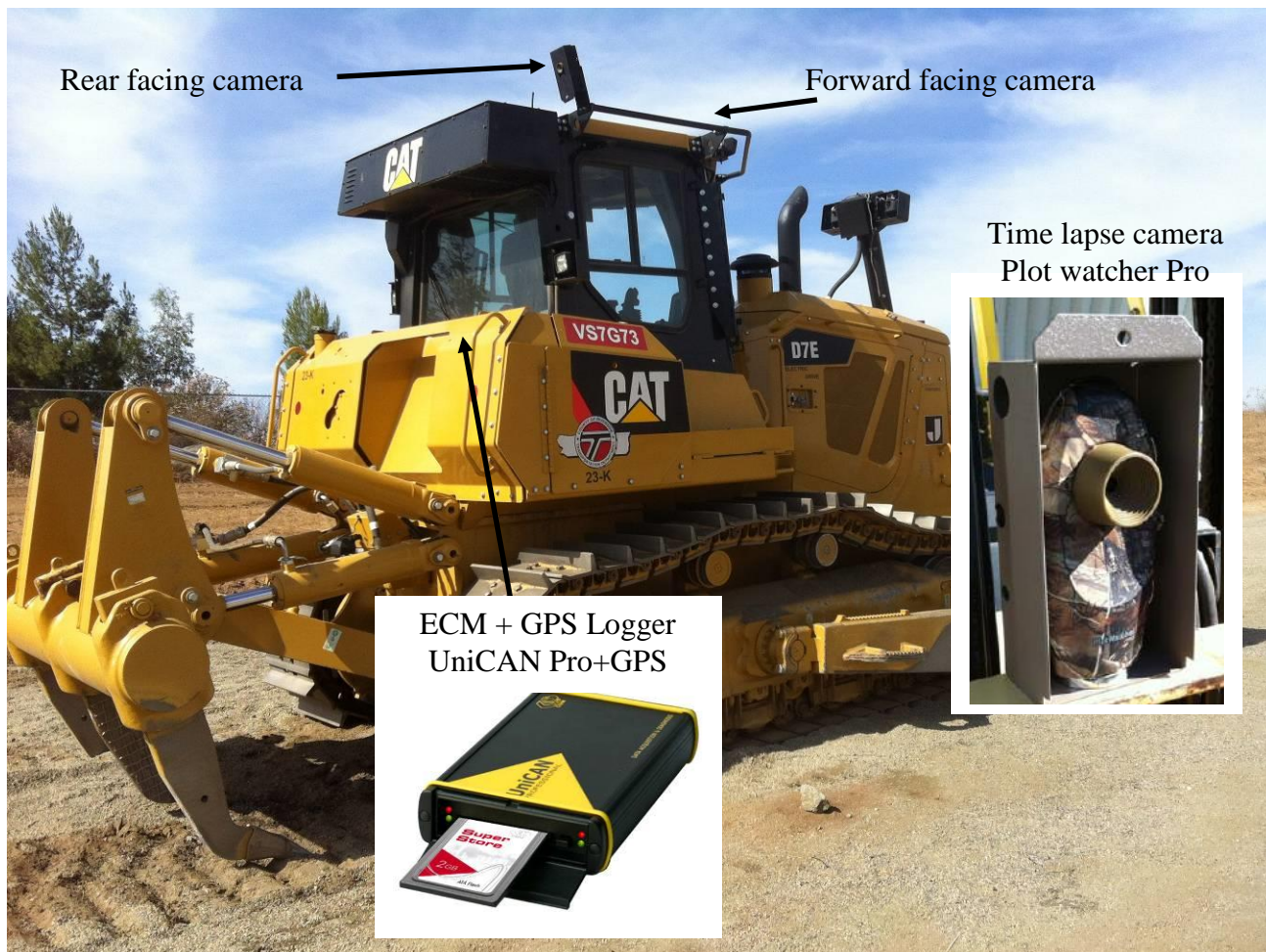
Figure 3-4 Activity measurement tools ECM, GPS, and time lapse video on the D7E
