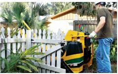
**SLENDER PROFILE DESIGN.** A 35.5" (90.2 cm) width makes the unit fit through tight areas and narrow gates.
