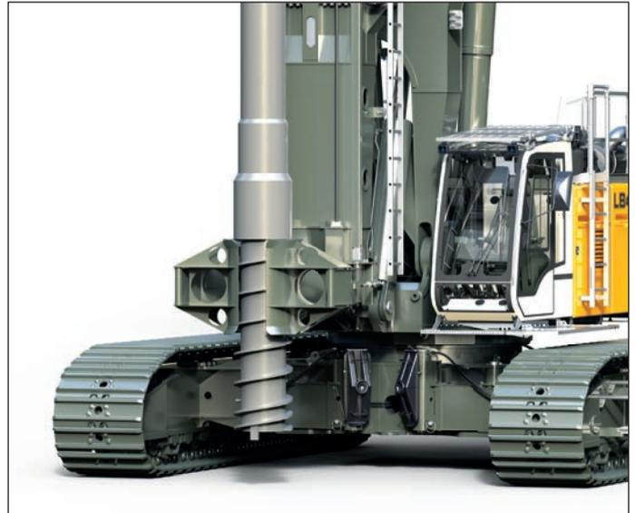
Full displacement tool with auger guide
