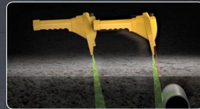
Holding the AML's handle parallel to the ground, scan the area of the suspected pipe or buried object until one or both of the AML's target indicators activate.
