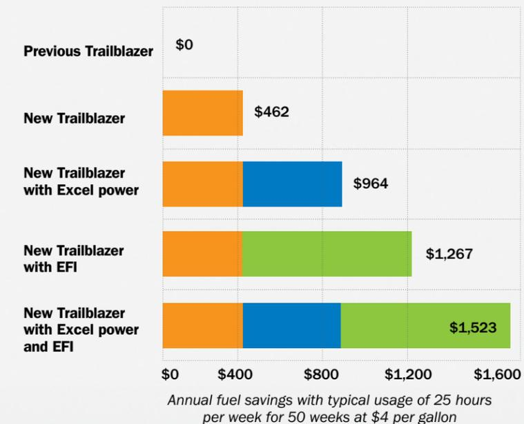
\* Estimated based on typical usage — 150 amps welding 40% of the time; 20 amps generator power 30% of the time; and idling without load 30% of the time.
