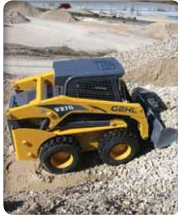
**EXTRA LONG WHEELBASE** of up to 55 inches (1387 mm) enhances machine stability when lifting and loading and provides a smoother ride over rough terrain.
