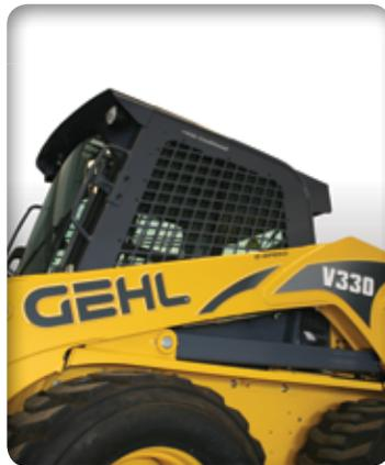
**EXCELLENT VISIBILITY** to the sides, rear and front is achieved with a unique, low-profile boom design. A roof window allows the operator to view the lift arm when in the fully raised position.
