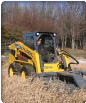
**AUXILIARY HYDRAULICS** are standard, powering many attachments. Optional high flow increases their capability. Dependent on control pattern, a rocker switch or foot pedal provides electronic proportional flow control.
