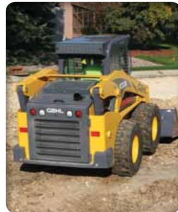
**HEAVY-DUTY CHASSIS** provides excellent weight distribution, enhancing machine stability. A rear bumper and counterweight on the model V330 add protection and towing capability.
