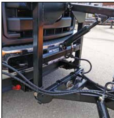
*Standard Medium-duty Quick Hitch: for use with MTP & MTP-Flex.*
