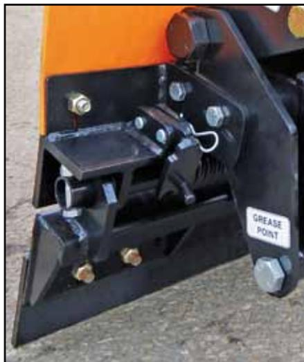
*Adjustable Trip-edge: (6) adjustable torsion springs.*
