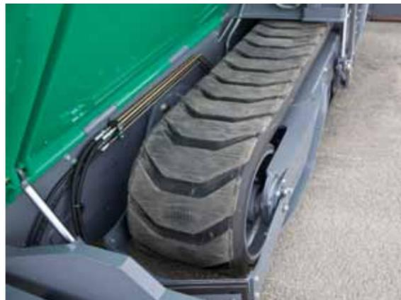
A strong point of the VISION paver is its excellent traction behaviour. Separate drive and electronic control provided for each crawler track ensure optimal transmission of power, constant straight-line tracking and accurate turns.
