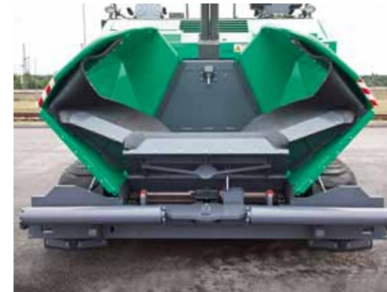
The hydraulically operated hopper apron prevents material spills during truck exchanges. It directs the material inside the hopper directly onto the conveyors, so no hand work is required. All of the mix is properly conveyed to the screed.
