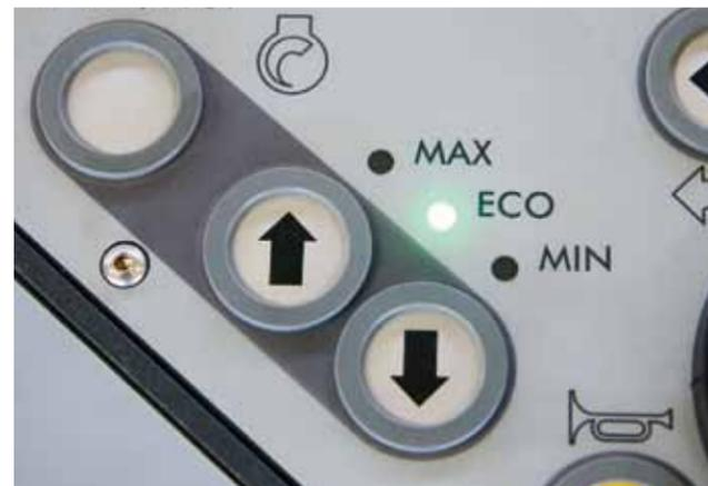
Three engine speed ranges are available which are selected conveniently at the push of a button (MIN, ECO, MAX).
