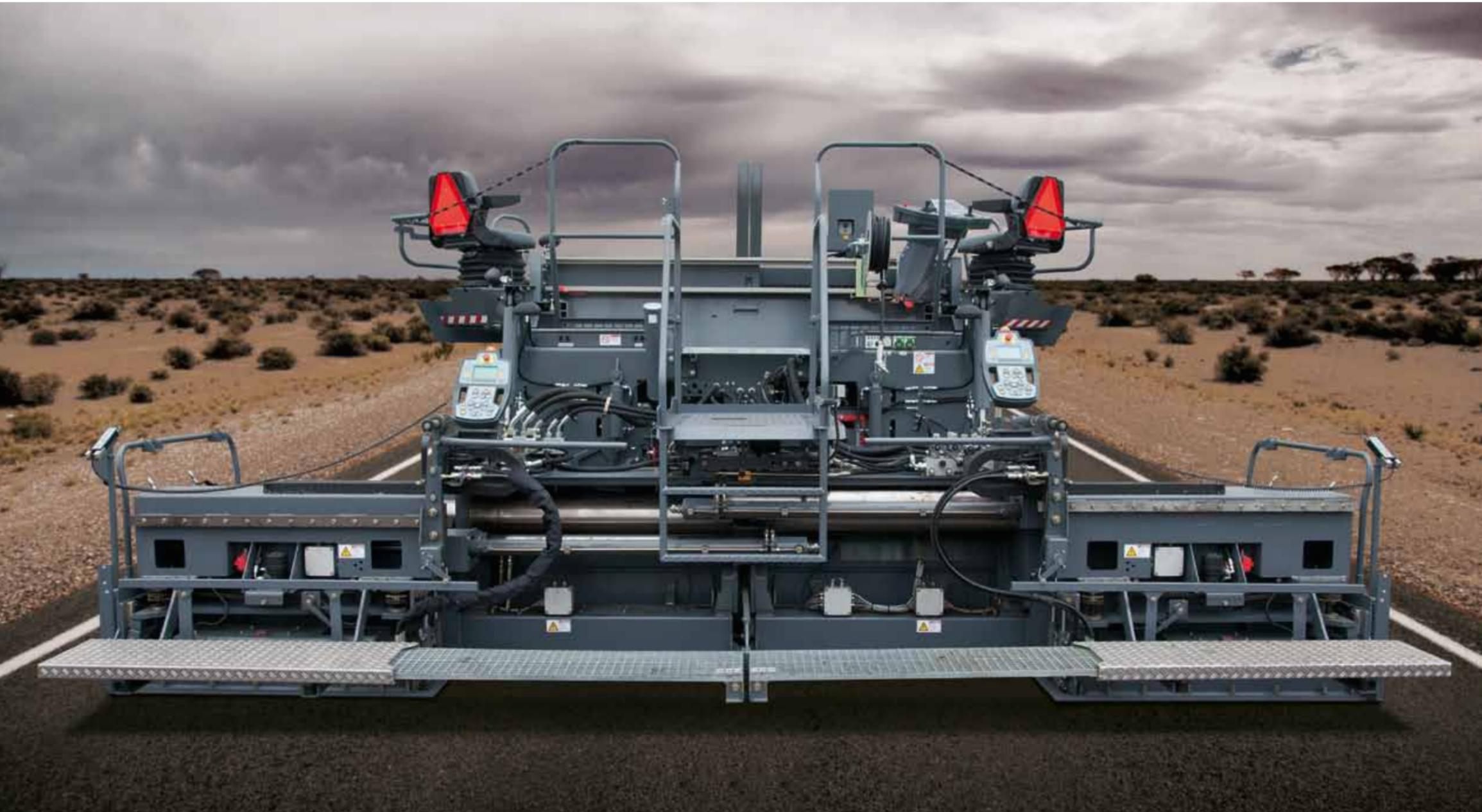
When paving across large widths, absolute accuracy of line and level is a crucial criterion for prime-quality results, regardless of the paving width and layer thickness involved. The new VÖGELE VR 600 Extending Screed boasts impressive abilities in this respect: its basic width is 10 ft. and it can be extended hydraulically up to 19 ft. 8 in. – to nearly twice
