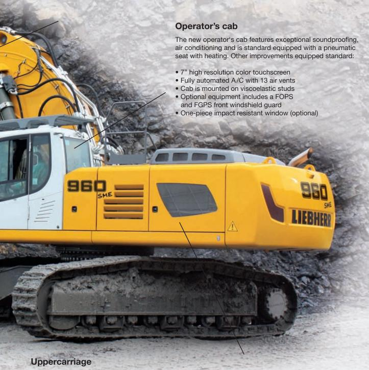
The uppercarriage has been designed to increase visibility to the rear of the machine. To improve this visibility even more and increase safety during movements, the machine is equipped as standard with a backup camera mounted in the counter-weight. Additional features of this uppercarriage are:
