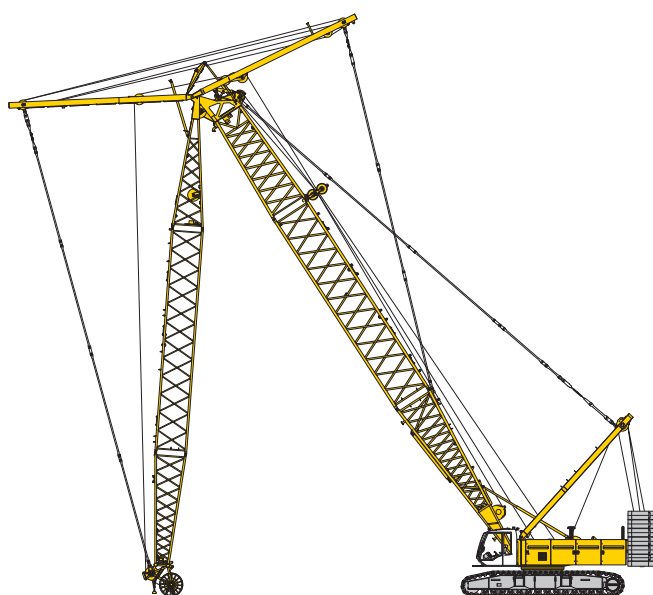
Erecting of main boom and luffing jib
