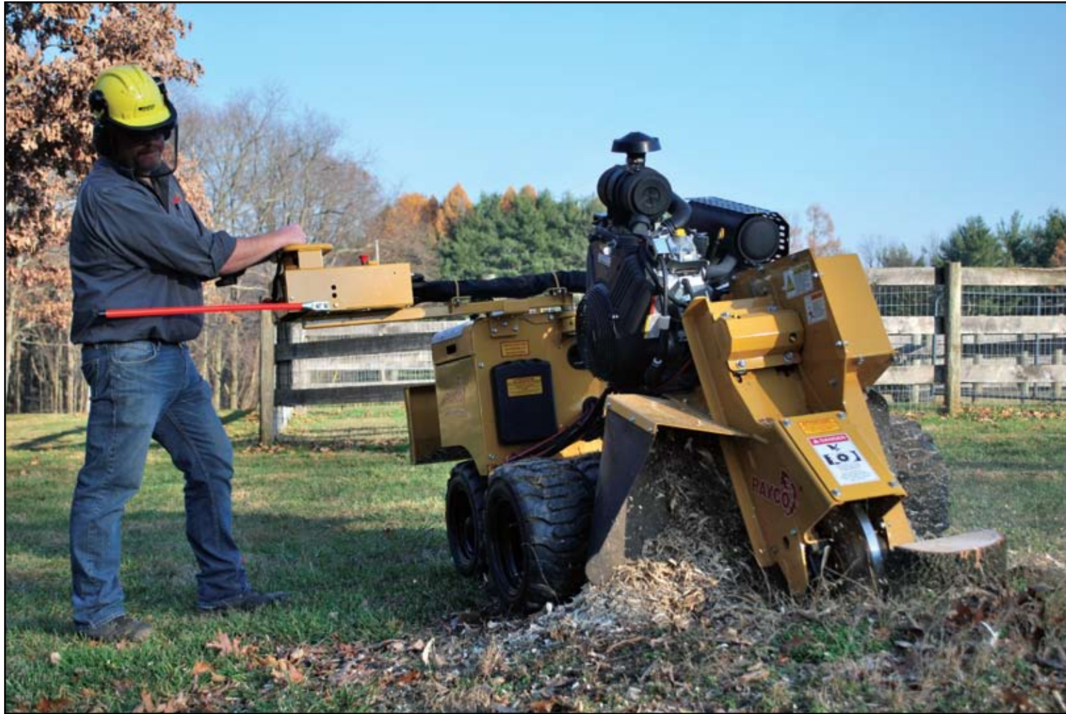
Swing-out controls for a better view of the cutting action
