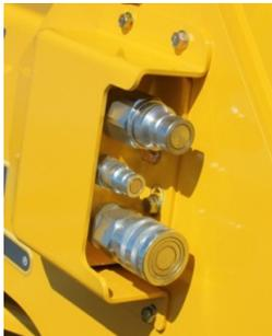
Auxiliary circuit incorporates pressure-relieving coupler block for fast, efficient attachment changes.
