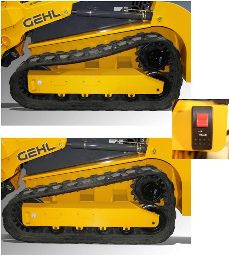
Reduce operating costs, save time and boost productivity with the industry-exclusive Automatic Track Tensioning System found on the Gehl RT250 Compact Track Loader.
