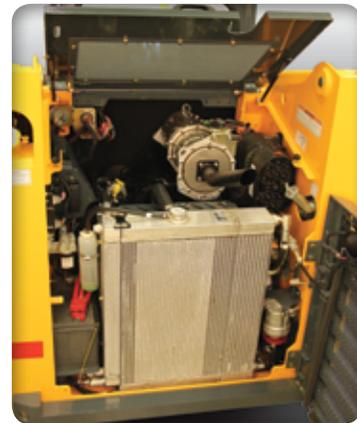
**SPEEDY SERVICE** is made possible with a swing-open rear door, flip-up engine cover, and tiltable ROPS/FOPS that fully exposes maintenance points at the engine, battery, and filler caps.
