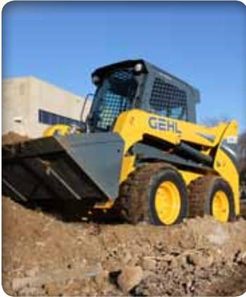
**STABLE RIDE** is achieved with a longer wheelbase and low center-of-gravity. The HydraGlide™ ride control option provides smoother operation over uneven surfaces.
