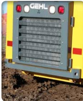
**COUNTERWEIGHTS** are optional and boost the rated load capacity to 2,110 lbs. (957 kg) on the R190, 2,370 lbs. (1075 kg) on the R220, and an impressive 2,780 lbs. (1261 kg) on the R260.
