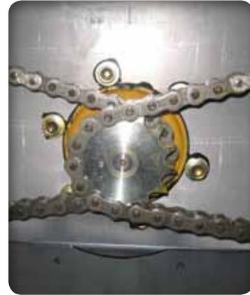
**HEAVY-DUTY DRIVETRAIN** is composed of durable components including zero-maintenance axles. Adjustments can be made to the chain system from outside the unit.
