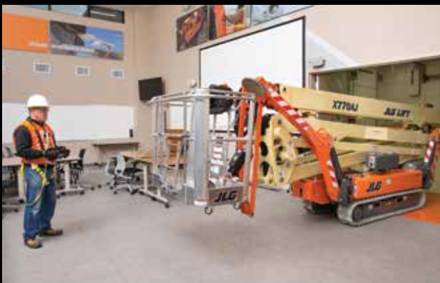
The X770AJ can go through double doors.
