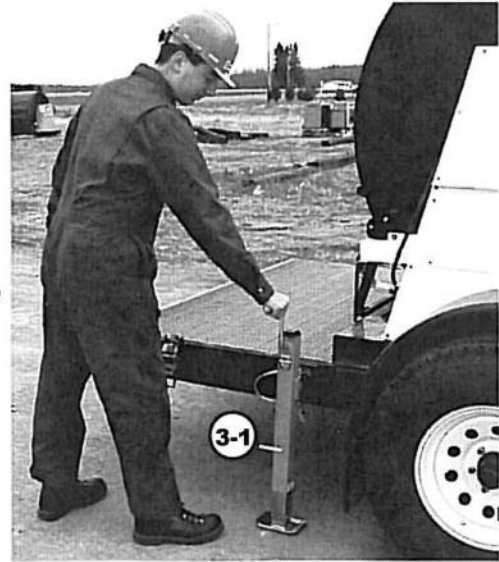
3 - Levelling & securing the trailer
