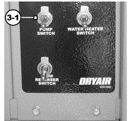
3 - pump, water heater & flow reverser switch
