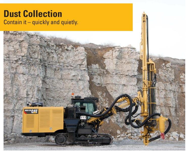
Powered to clean holes up to 152 mm (6 in), the MD5150 dry dust collection system is efficient, quiet and it consumes less power than traditional dust collectors. The heavy-duty system effectively manages rock fragments and dust yet is also easy to clean and service.
