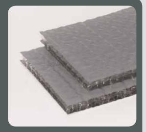
Closeup of insulation blanket construction showing two layers of closed cell insulating pockets protected by two outer reflective layers.
