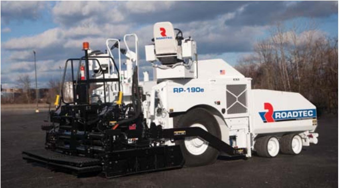
The RP-190e is a powerful, heavy-duty rubber tire paver for highway work offering operator comfort and safety with 360° visibility, fingertip controls, fully adjustable seats, low noise levels, and fume extraction systems. The exclusive Roadtec anti-segregation design gives consistent pavement quality. Dependable and tough.
