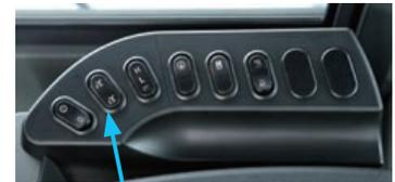
Dual mode engine power selection switch
