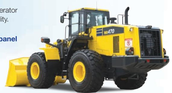
**Remote boom and bucket positioners** can set kick-outs from inside the cab.
