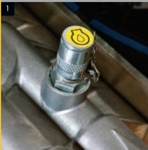
1. Fluid-sample and diagnostic test ports simplify preventative maintenance work and troubleshooting.
