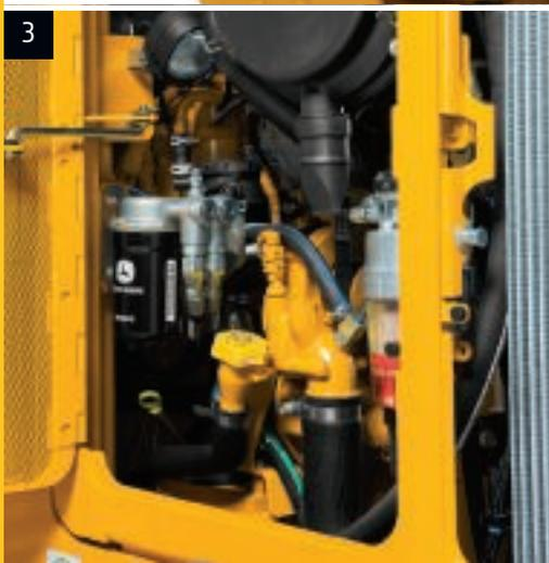
3. Large service doors open wide, and same-side daily checkpoints are conveniently grouped for ground-level access. Engine, hydraulic, and coolant checks and refueling can be done quickly without climbing on the machine. Plus, an under-hood light helps show the way.
