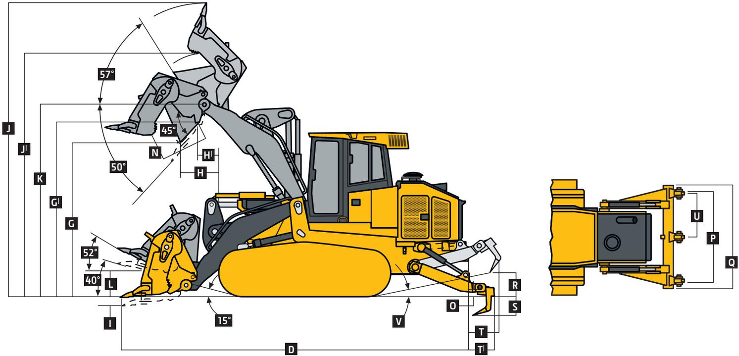
655K CRAWLER LOADER WITH MULTIPURPOSE BUCKET AND 3-SHANK RIGID-TYPE RADIAL RIPPER WITH ESCO RIPPER TIPS
