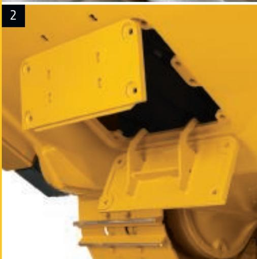
2. Hinged butterfly-style belly pan folds down, providing easy service access to the oil pan.
