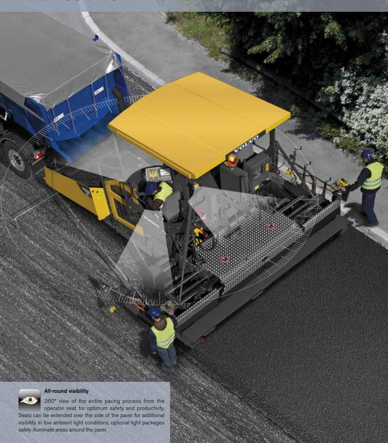
Step onto the operator platform and admire your work from 360°. Observe continuous material flow from the large hopper, which holds enough material for continuous paving. See the uniform delivery of material in the auger channel as the conveyor and augers work perfectly together to provide a seamless, smooth mat.
